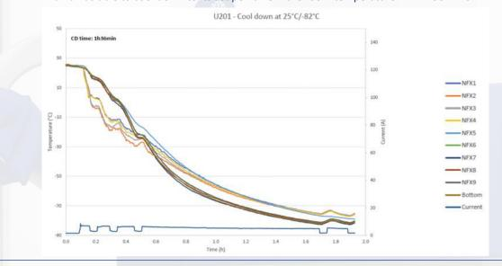
The testing was conducted at 25°C ambient with a set point of -82°C (unloaded condition) 1.
